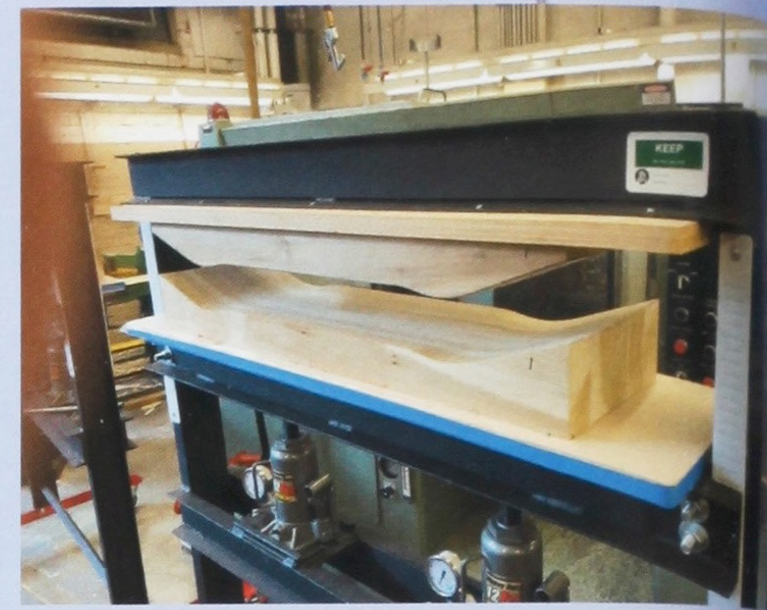
Creating a skateboard deck starts with the forming of the wood in a press. Students learn how to design, press and complete a unique skatedeck in this class. Casting the trucks comes next.
