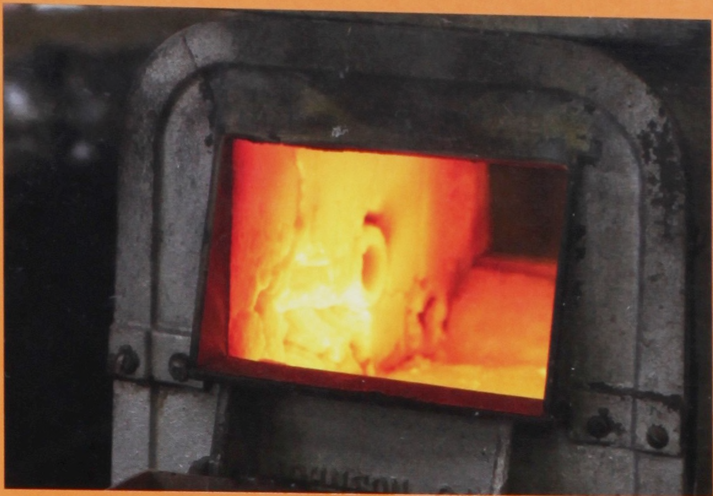
The forge is seen here, used for generations of manufacturing students to make the iconic screwdriver. This thing gets hot, at about 1800°F this thing will make the steel "plastic".
