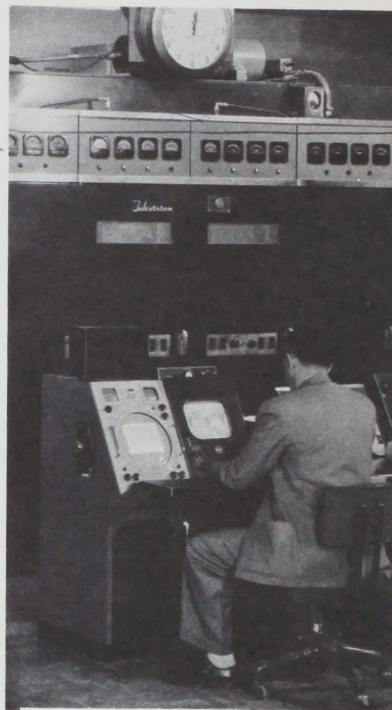
Shown above is monitoring board at transmitter building. Photos compliments of station KPTV.
