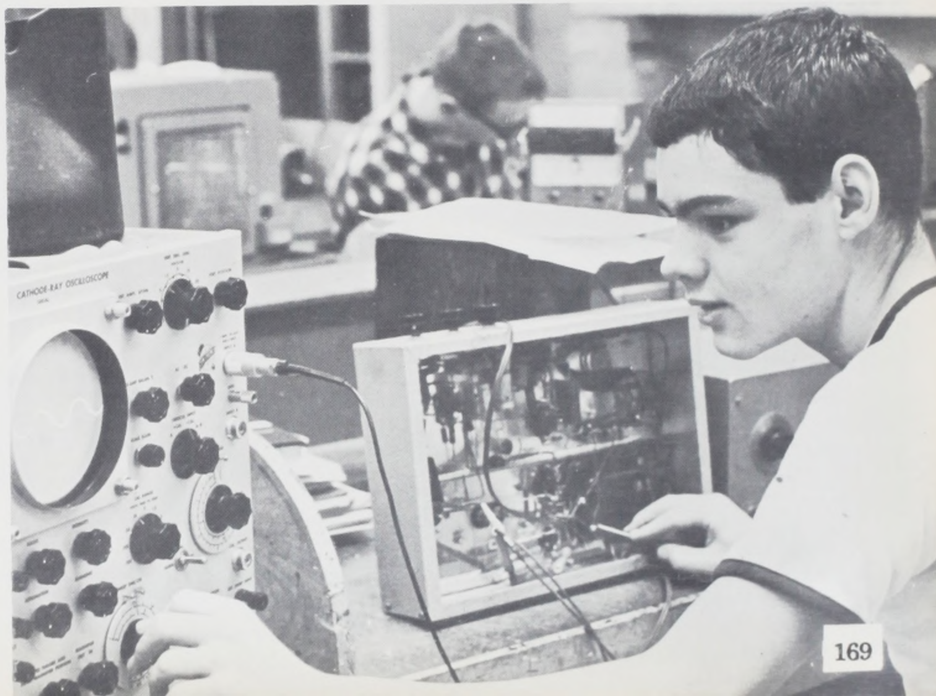
Lanny Coate, senior radio major, built this amplifier in the shop. Here, he tests his creation on one of the new oscilloscopes to trace the signal through out the amplifier.
