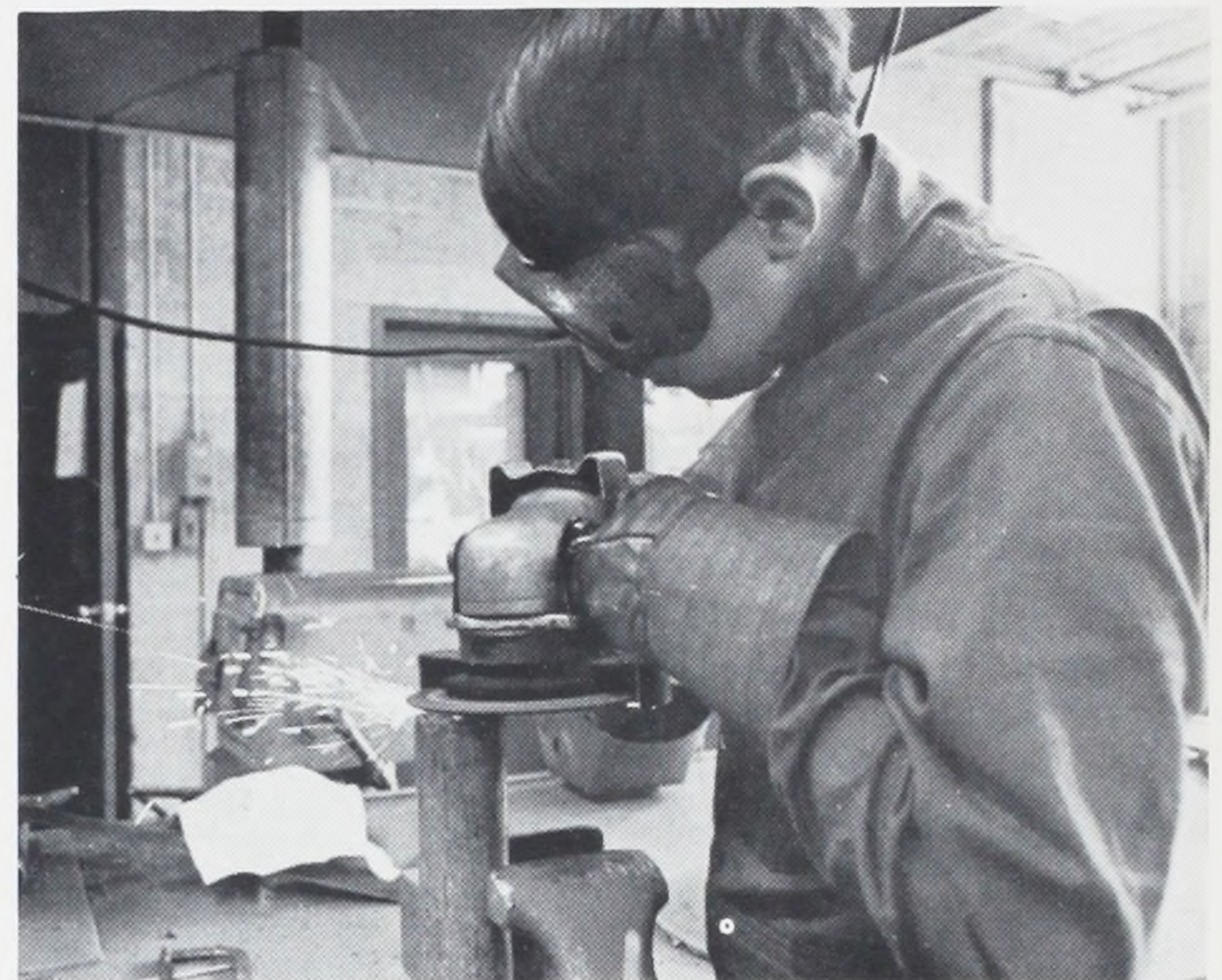
Mark Weidner uses disc sander with a weld-cutting disc-plate to practice cutting a weld.
