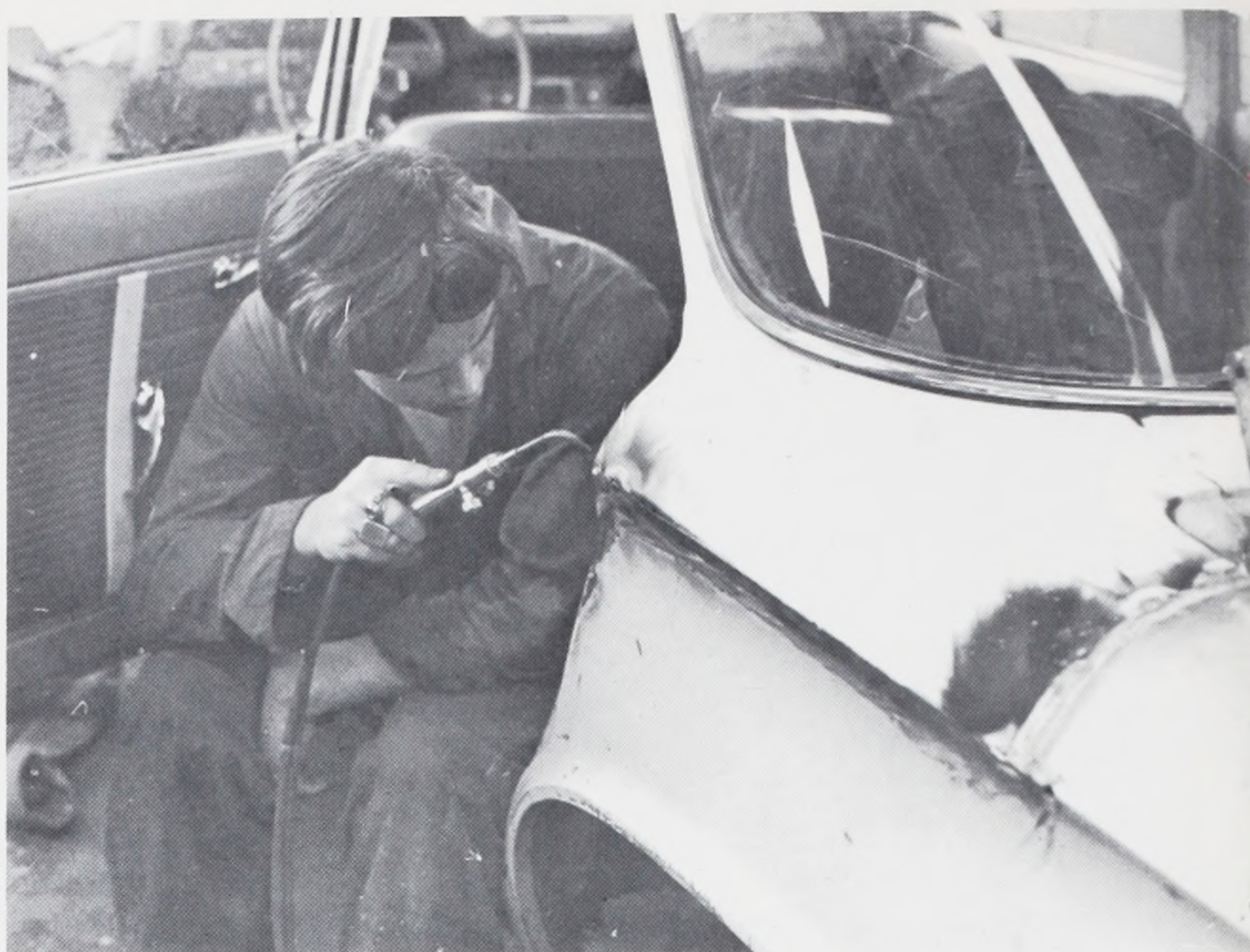
Senior Body and Fender Automotive major Mike Brady uses Acetylene torch to weld fender on Corvair. Body and Fender is taught by Mr. Theodore Raisig.
