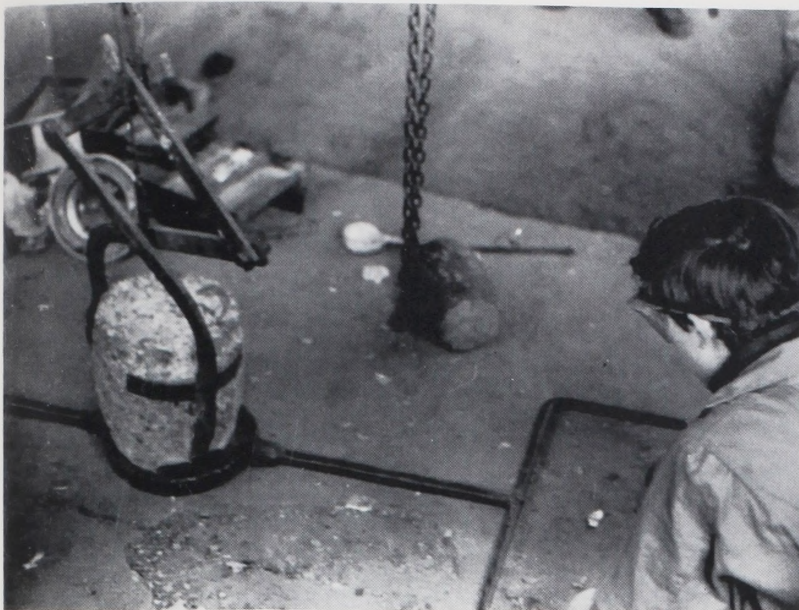
Student in Foundry lifts crucible out of furnace.
