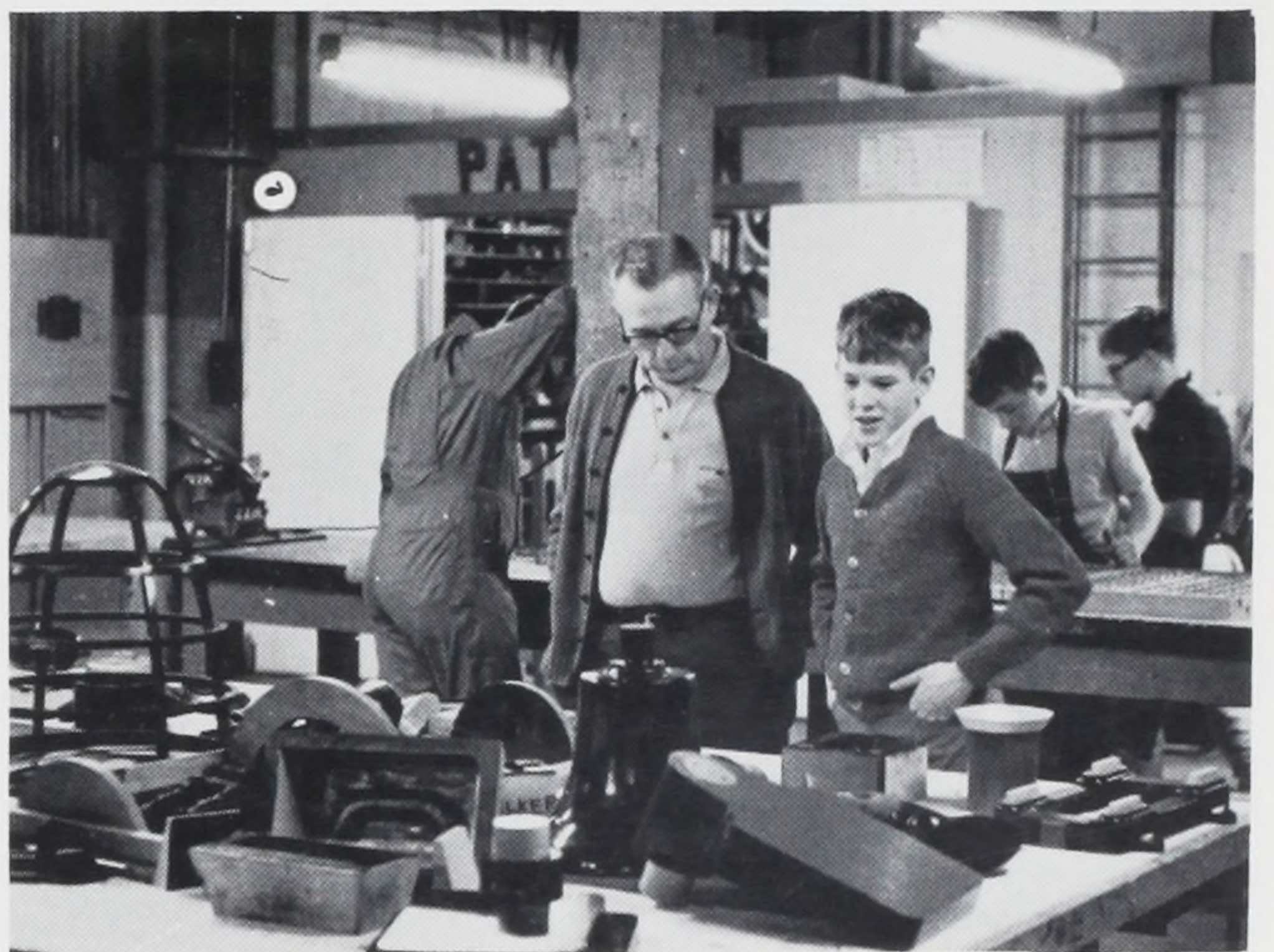
Father and son view wooden patterns made in pattern shop for use in foundry.
