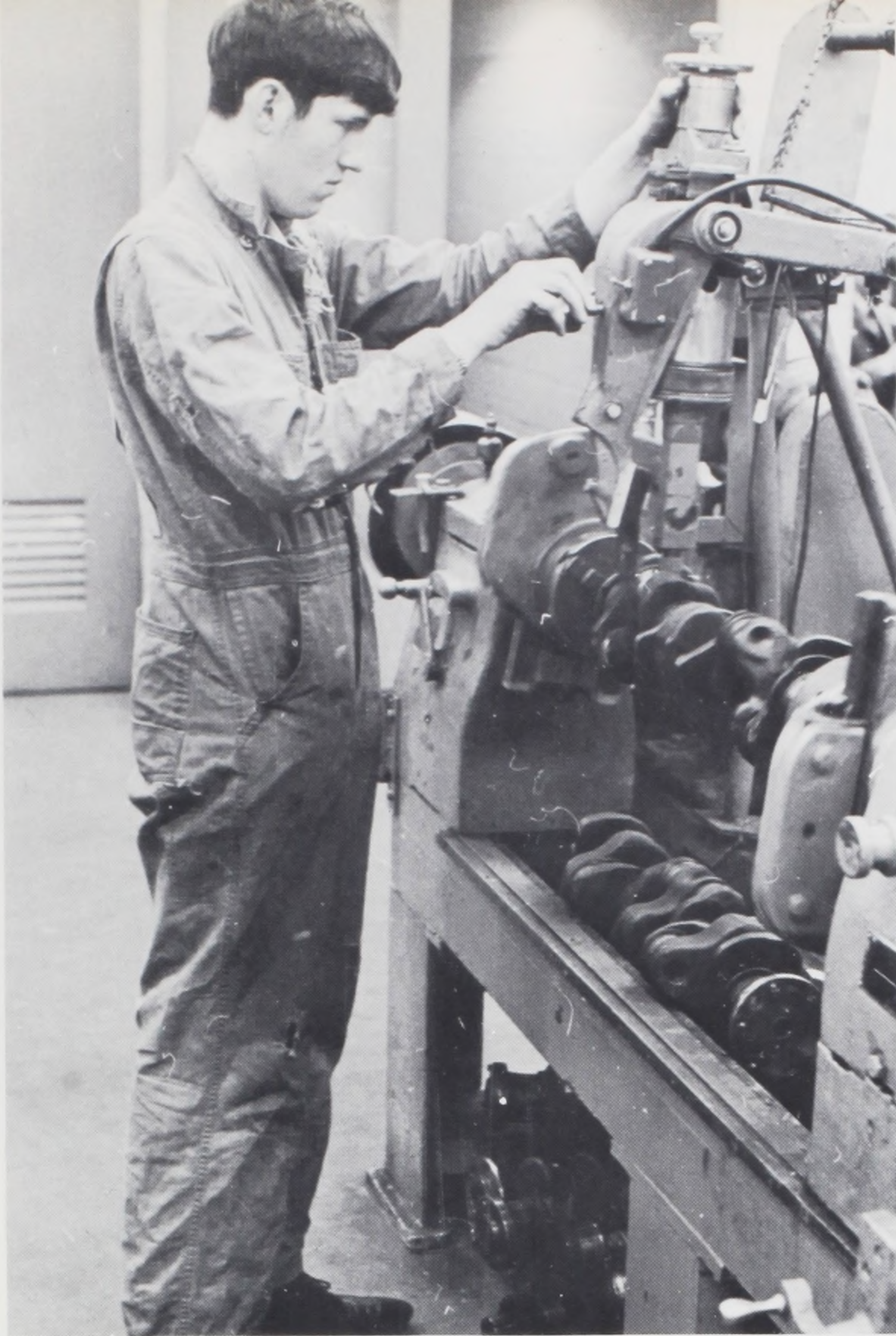
Clockwise, from below: Kim McComb dismantles brake-drum; Dave Rogers and Mike Gregory buddy up in checking a motor; Bill Shipps removes a fuel pump; Don Gilbertson and Dan Dittler bore a fly-wheel; Allan Bronson and Bill Shipps check a motor; Dave Hoard reshapes a crank shaft.
