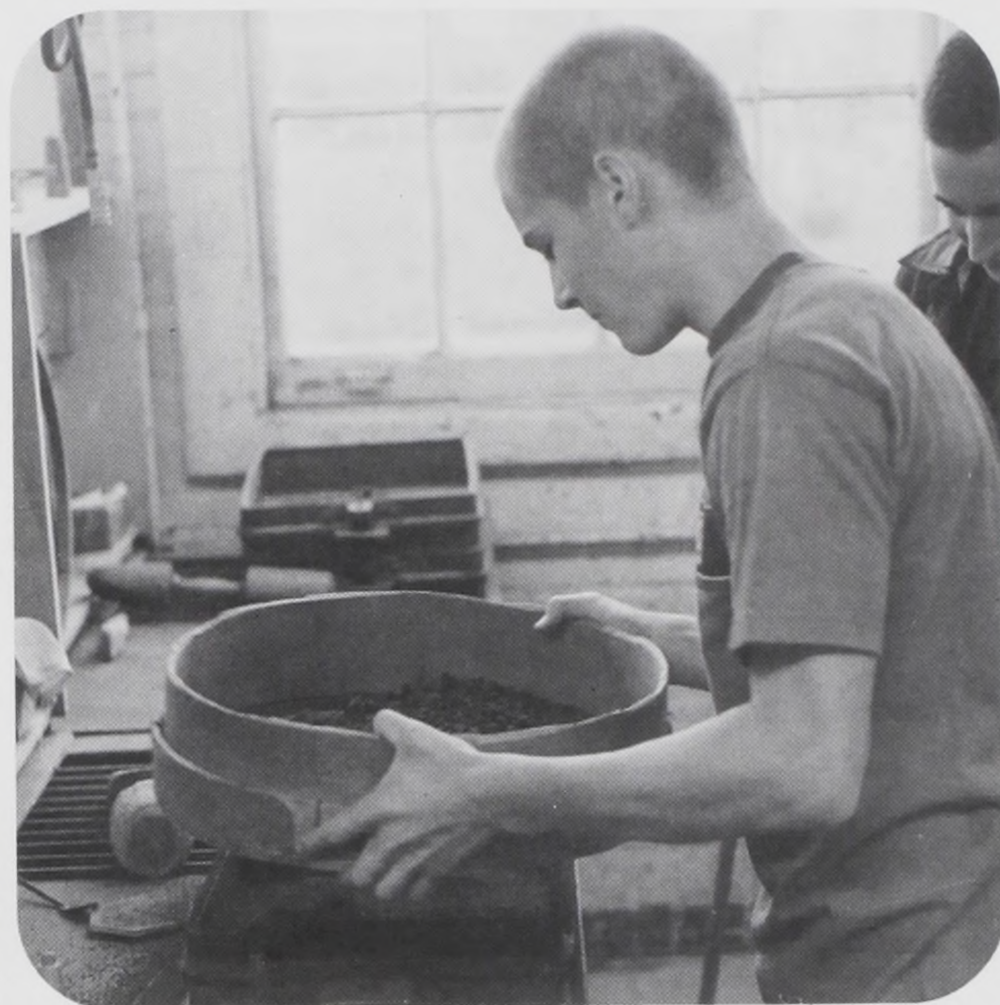
Nathan Turner extracting big pieces of sand from the moulding clay
