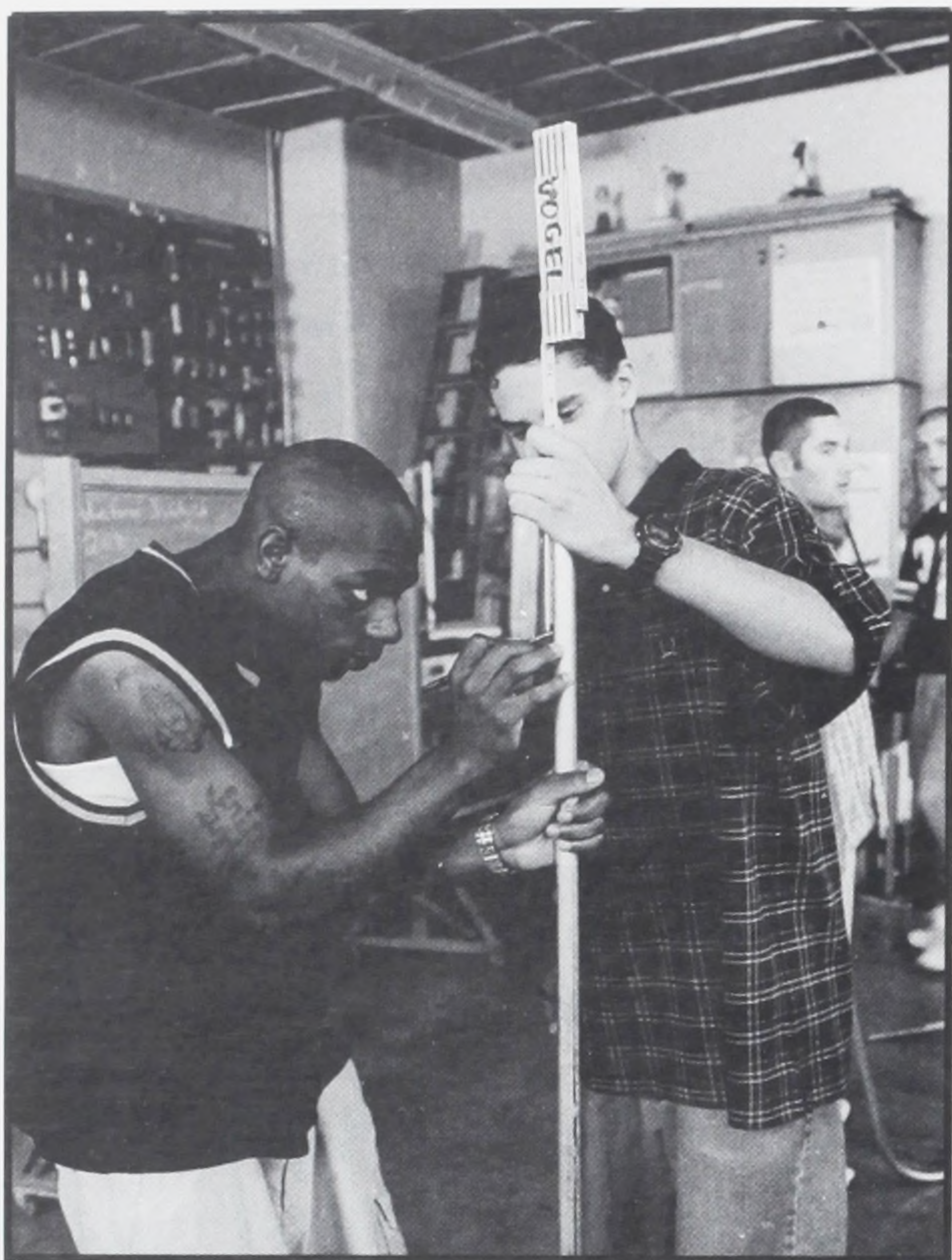
Myron Clark and Nick Trujillo measure conduit for bend.
