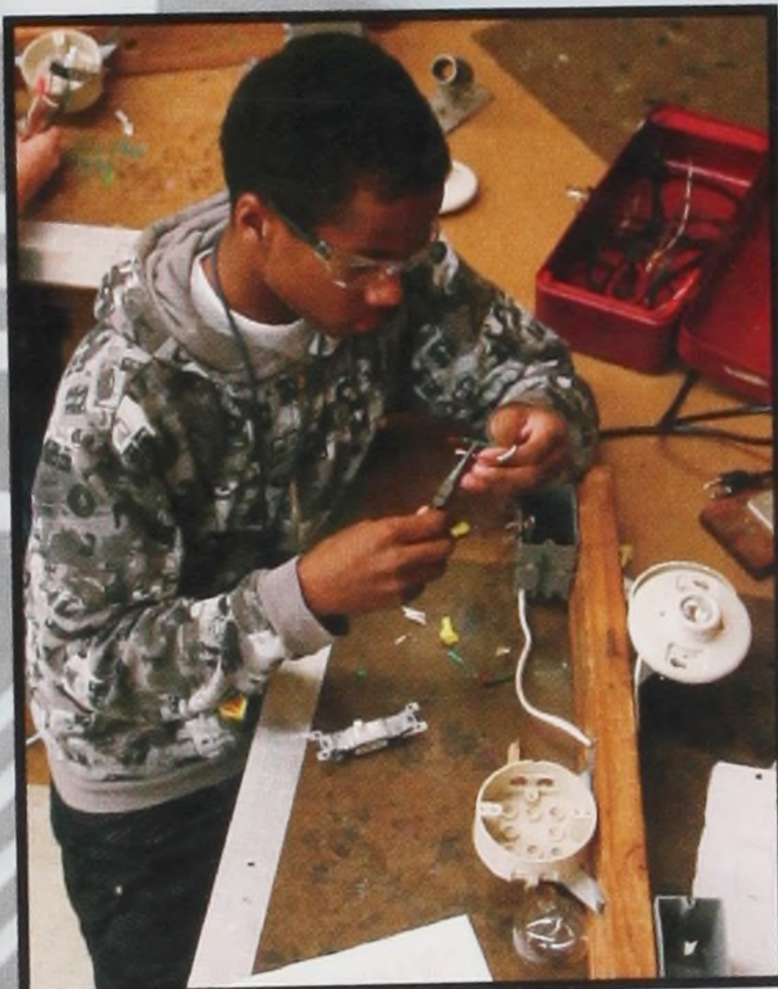
Blair Tinker strips wires for use in his projects. The wires are covered by insulators to prevent fires from starting. Some of it has to be cut to leave some actual wire out to work with.
