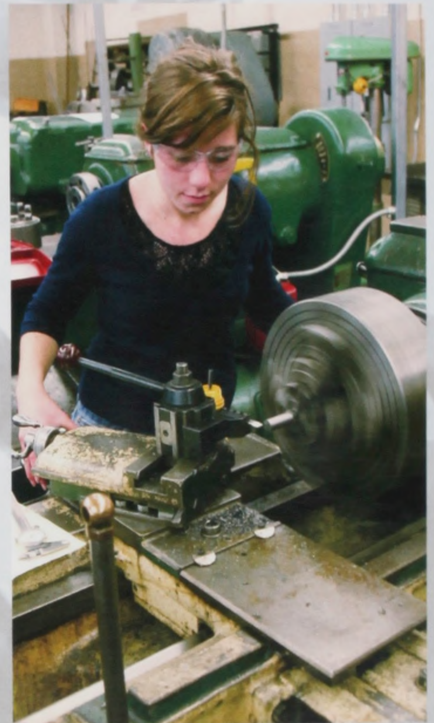
Right: Breanna Burnside turns a ramp piston for her hydraulic jack.
