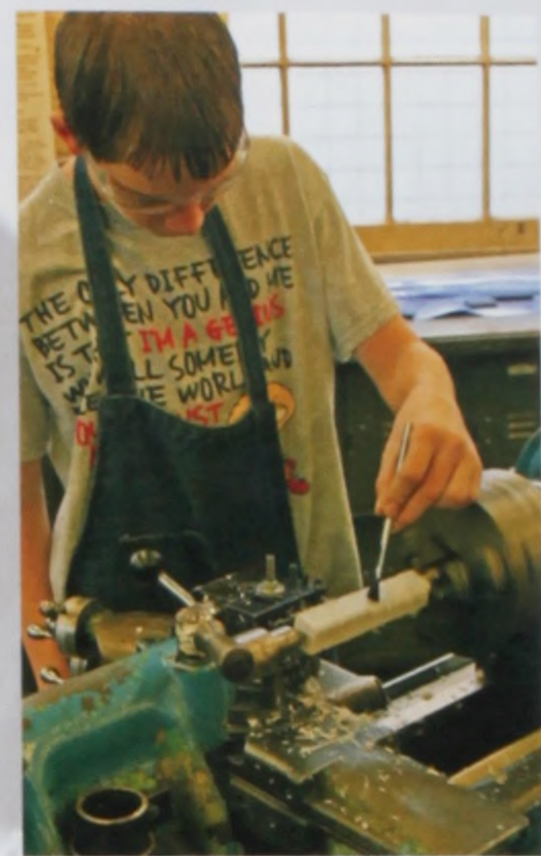
Top left: Hunter Ruttum uses the lathe to craft a pump piston for his hydraulic jack project in Senior Manufacturing.
