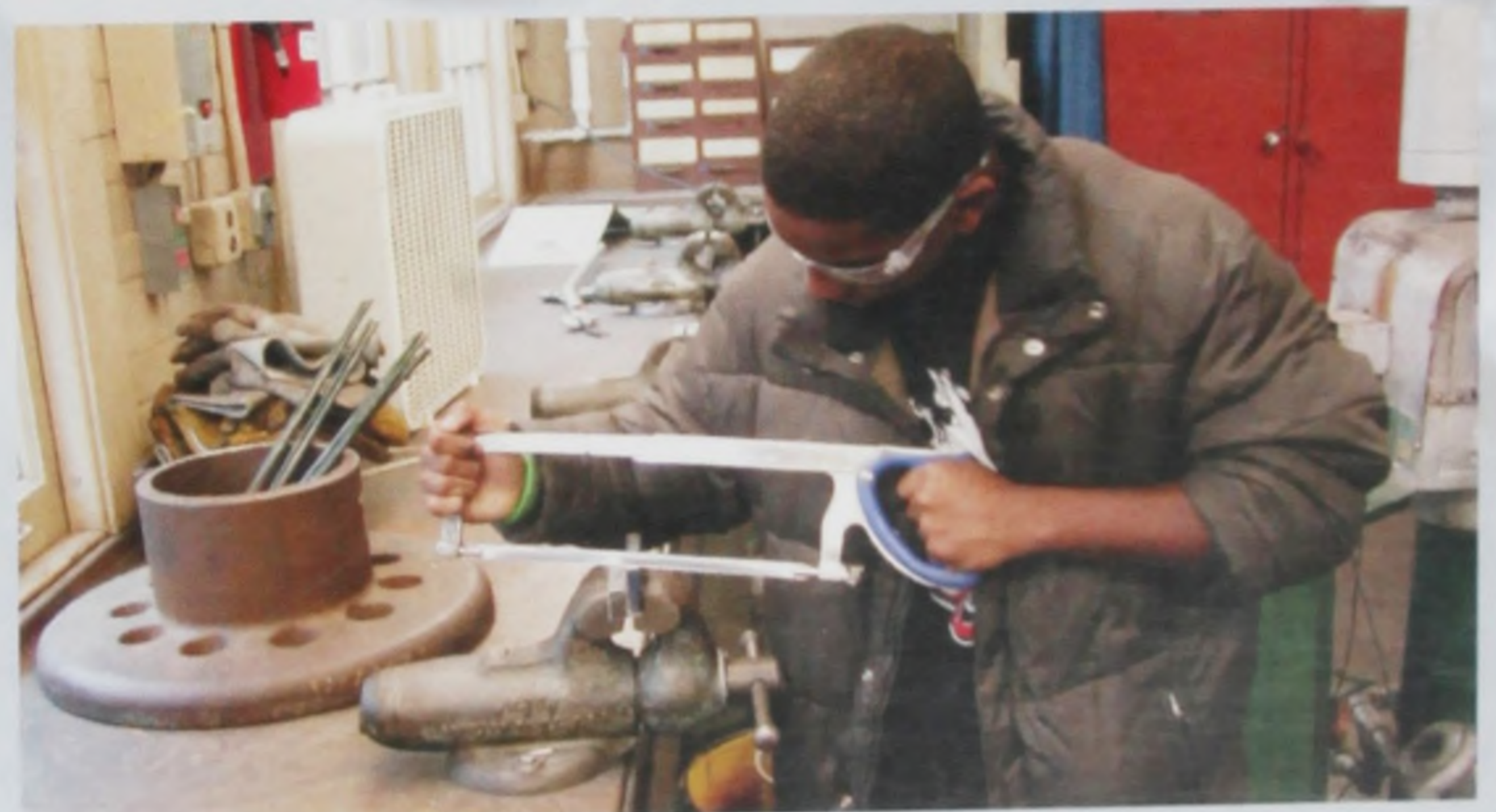
Below: Kavonte Rice saws the corners off of his C-Clamp to prepare it for the shaper.
