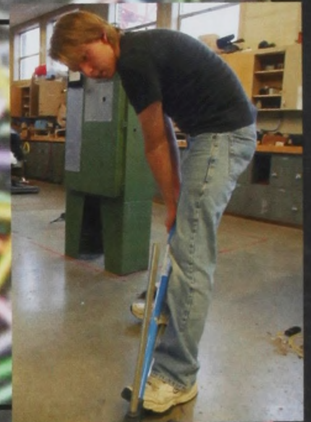
Senior David Remington bends conduit in preparation for laying down electrical wire.
